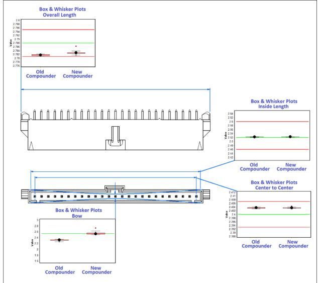
4.4 Conducted trial assembly runs with housings run with resin from both compounders
